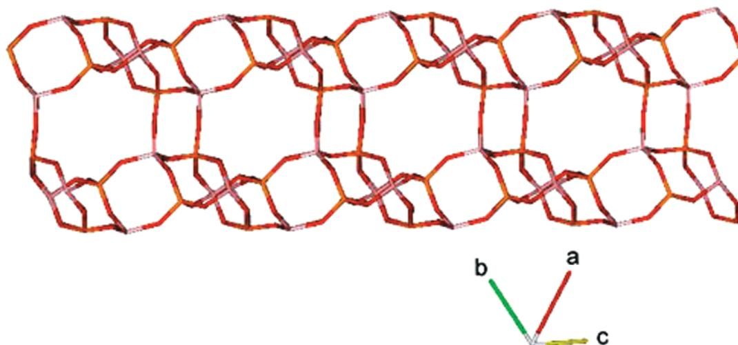
**Figure 6.** The 8-membered rings channel along the crystallographic [111] direction in  $\text{BePO}_4\text{-GIS}$ .
