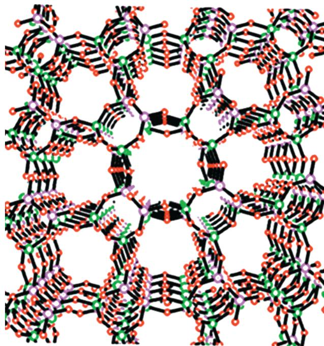
**Figure 5.** The 4.8.8 network of strictly alternating  $\text{BeO}_4$  and  $\text{PO}_4$  tetrahedral in which all the vertices have a shared viewed down the  $c$ -axis in  $\text{BePO}_4\text{-GIS}$ .
