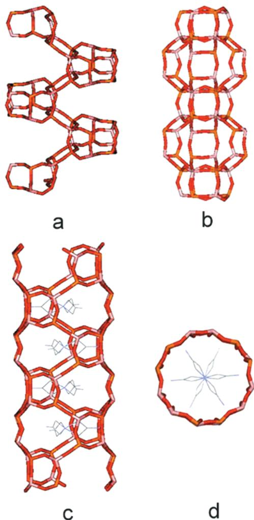
**Figure 4.** Subunits of  $\text{BePO}_4\text{-GME}$ : (a) the ABB sequence of double 6-membered rings, (b) the  $[8^3 6^4 4^2 4]$  cage of  $\text{BePO}_4\text{-GME}$ , (c) the 4.8.8 net for  $\text{BePO}_4\text{-GME}$  along the  $c$ -axis, and (d) the 12-membered ring channel occupied by triethylene tetramine molecule, C2 atoms has two orientations.
