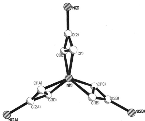
**Figure 8.** Two possible orientations of triethylene tetramine molecules in  $\text{BePO}_4\text{-GME}$ .
